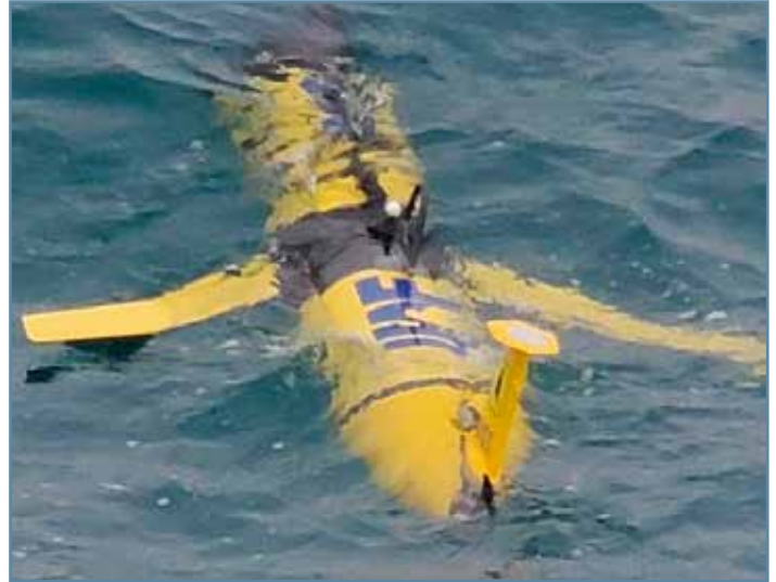
The Shackleton, an autonomous underwater glider being used to research Pacific Herring in Prince William Sound. Photo from the Prince William Sound Science Center.
