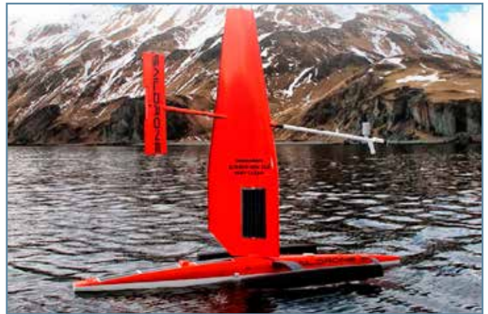
One of three saildrones used to acoustically survey Walleye Pollock in the Bering Sea in 2020. Photo by Saildrone, Inc.
