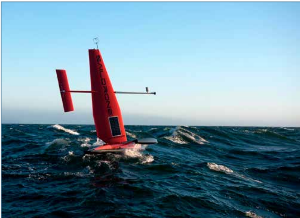
Saildrone to be deployed in the Bering Sea to track Red King Crab tagged with acoustic tags. Photo from Scott Goodman, BSFR.
