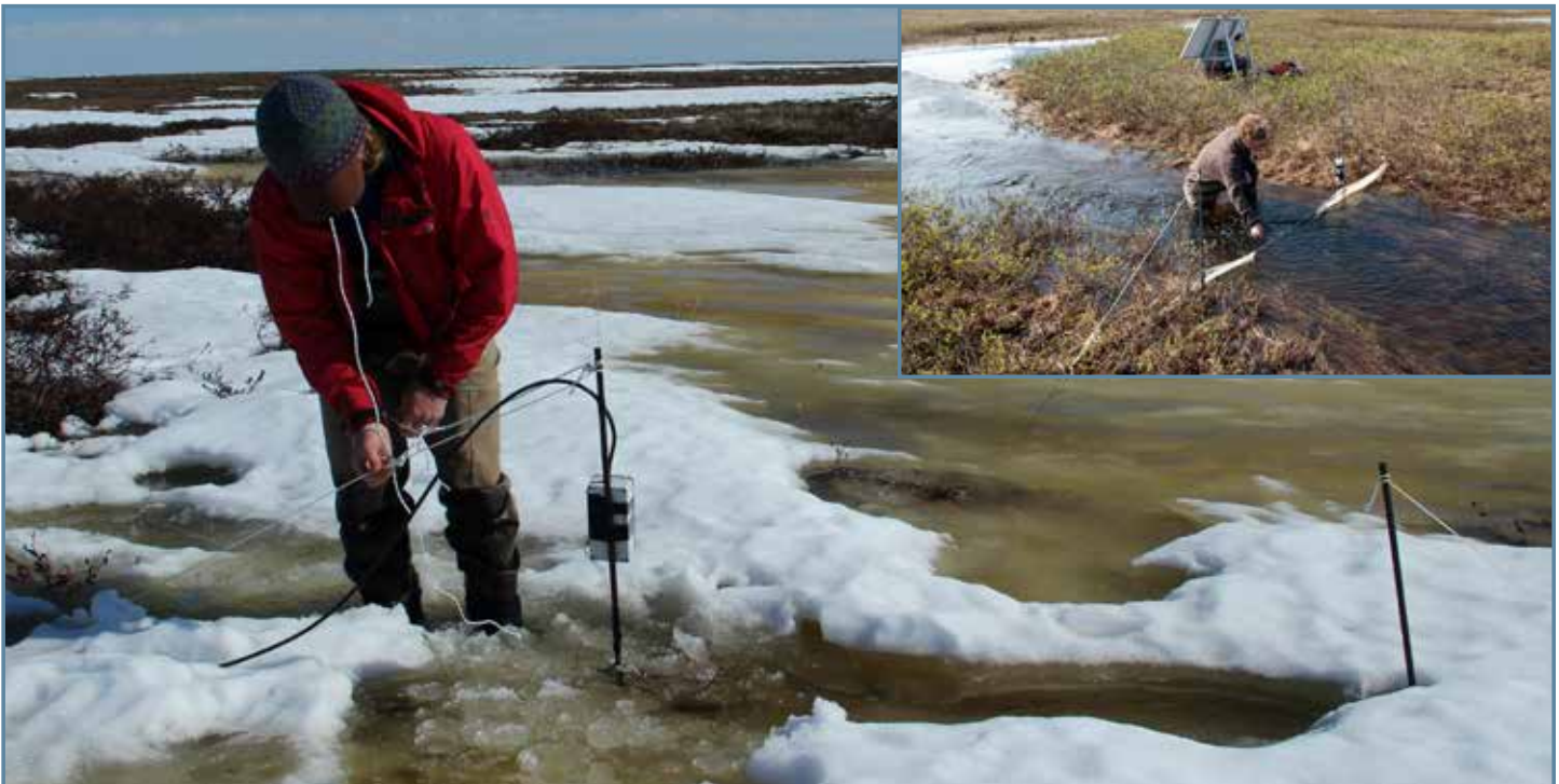
Stream-width PIT tag antenna in May 2013 set up while Crea Creek was still frozen, and in June 2013 (inset) after break-up. Photo by Lauren Flynn.
