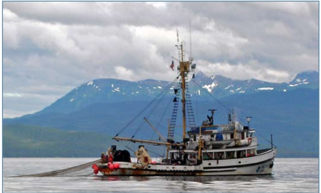
NOAA vessel J. N. Cobb trawling for epipelagic fishes in Icy Strait, 2005, with a 264 Nordic rope trawl.
